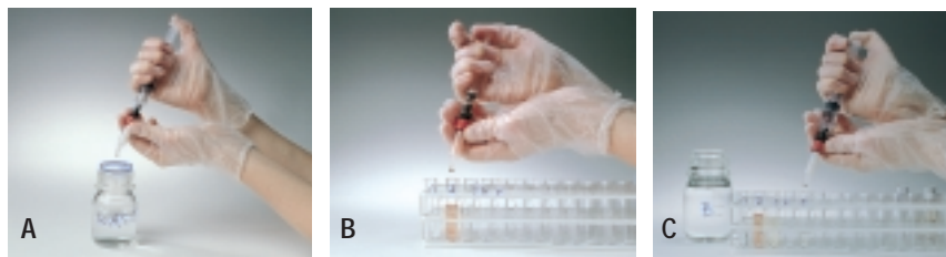
Fig. 3. Using GSTrap FF with a syringe. A Prepare buffers and sample. Remove the column's top cap and twist off the end. B Load the sample and begin collecting fractions. C Wash and elute and continue collecting fractions.
