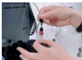
Connecting the column.
